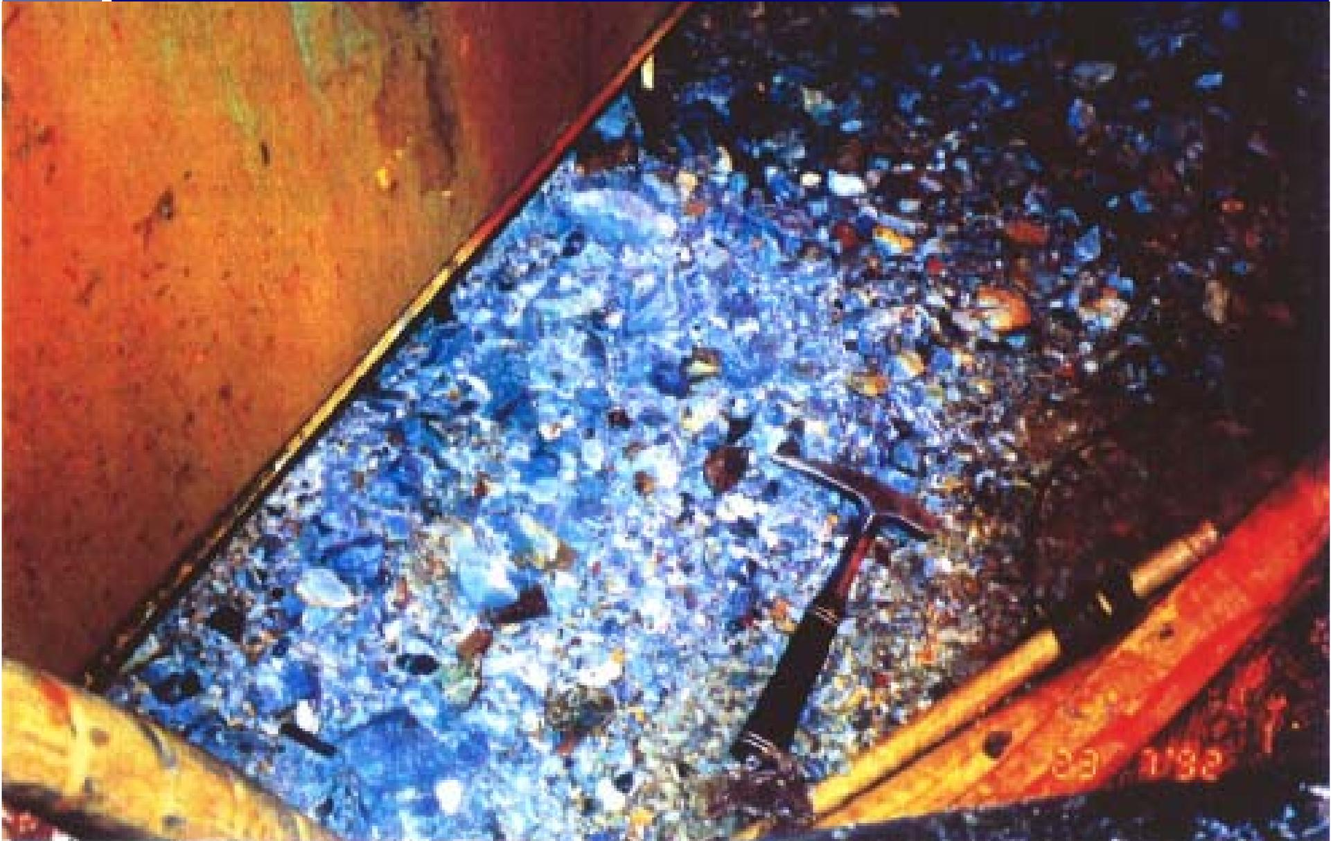
Angular pieces of quartzite and phyllite ejected from the HRT spring at chainage 1194
