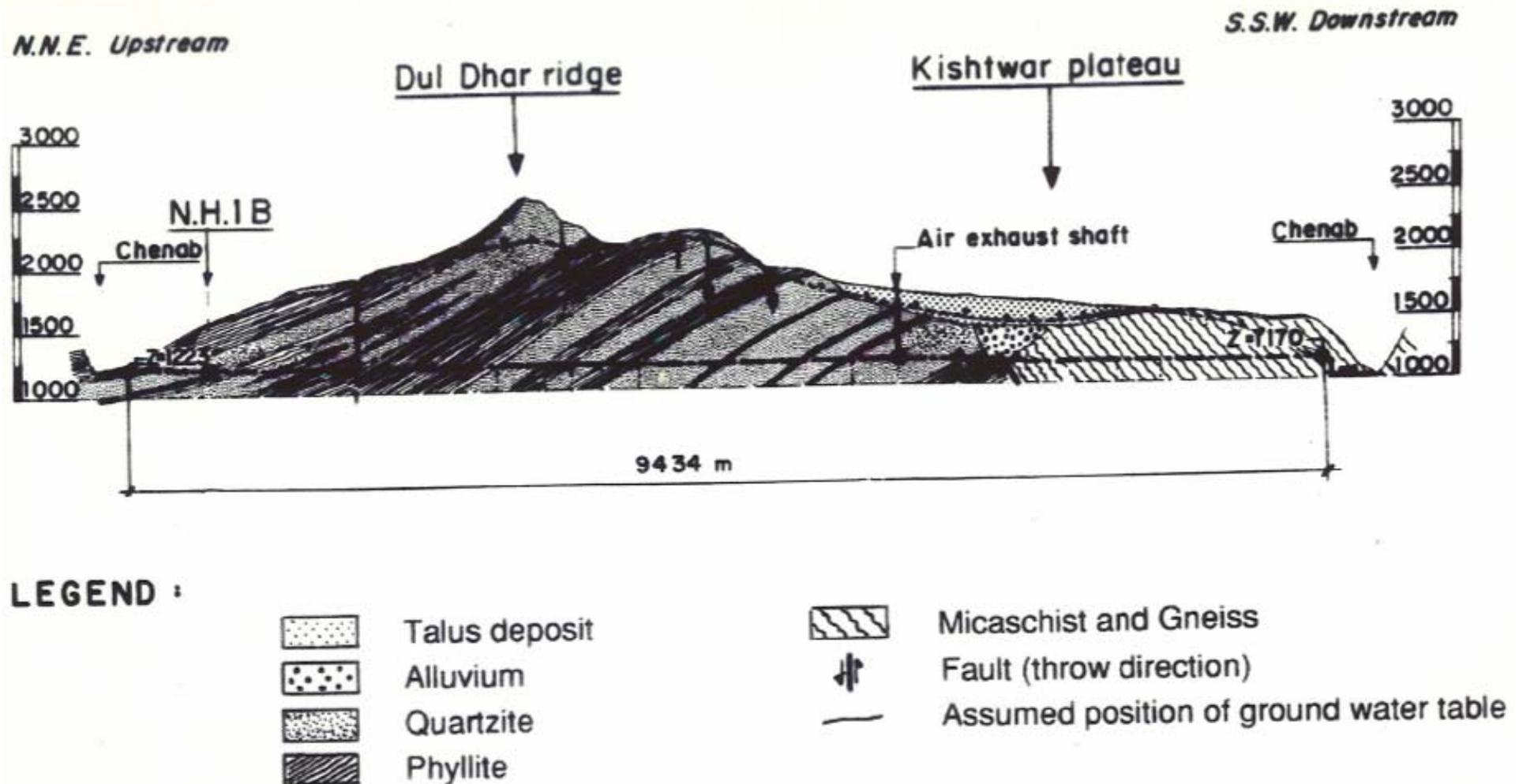
Fig. 4. Geological cross-section along the initial straight alignment of the tunnel, as known in September 1989.
