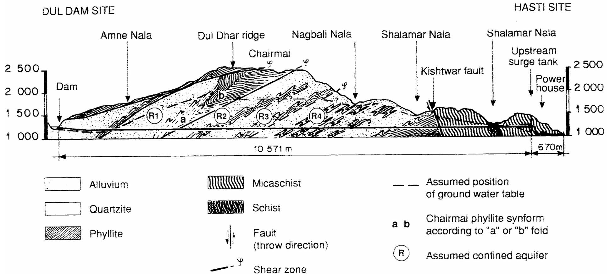
Fig. 16. Probable schematic geological cross-section along the final headrace tunnel route ("loop alignment").
